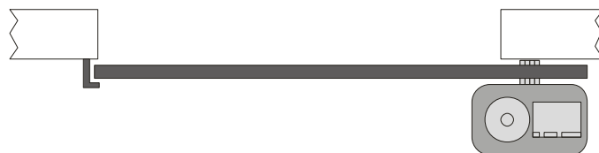
MC4 to the right DIP 8 is ON
